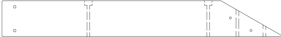
SB02 | SWING BEAM 2 POSITION - W4L15692 (x1) | 2"x5 1/4"x41 1/8" (50x134x1043)
