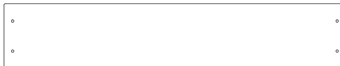
K01 | GROUND BOARD - W4L15672 (x2) | 5/8"x5 1/4"x27 3/4" (16x134x705)
