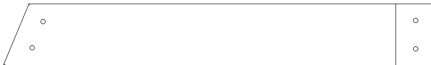
G03 | GROUND BOARD - W4L15697 (x4) | 1"x5 1/4"x36 7/8" (24x134x936)
